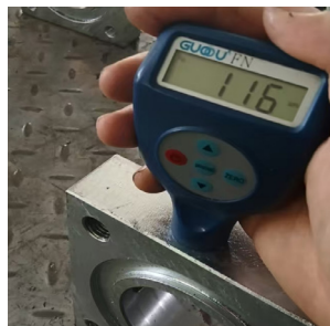
Hot Dip Galvanized thickness test
